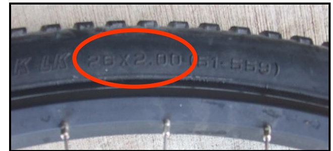
Examples: 26" Wheel Diameter & 2" Tire Width
