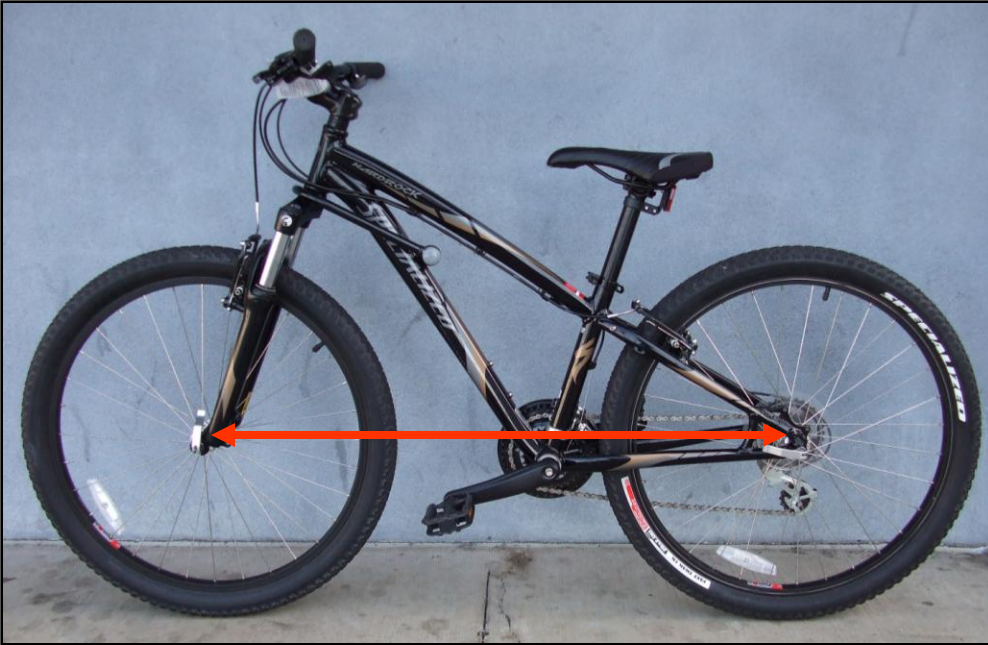
Examples: 26" Wheel Diameter & 2" Tire Width
