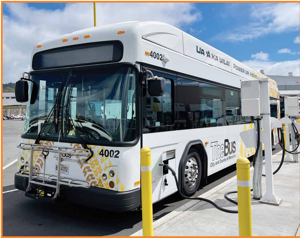
Photo above: The Gillig Electric Bus at the Kalihi-Palama Facility Charging Station
